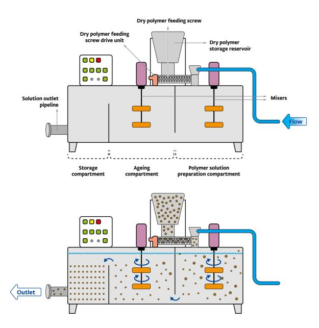
Dry polymer which is stored in the reservoir is dosed to the eductor. Water also enters the eductor, mixes with the dry polymer, and directly flows through the tank. The solution in the polymer solution preparation tank is mixed by a flash mixer. In the ageing compartment, the low-speed mixer keeps the polymer suspended. After these processes, the solution is stored in the storage compartment.
